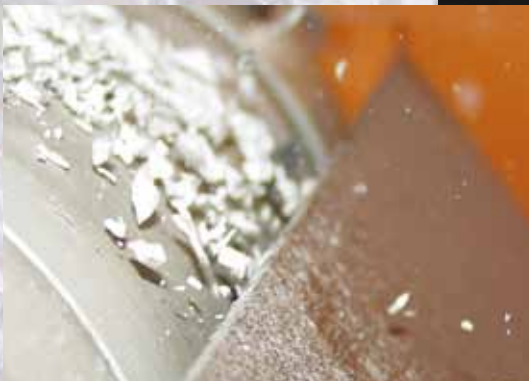
Separation of very small (sub 5mm) aluminium chips from plastics
